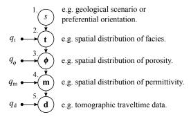
Figure 4.1: Graphical model for the proposed Bayesian hierarchical model. *s* stands for the structural parameter, t is the field of geological facies,  $\phi$  is the field of a physical property, m is the field of a geophysical property, d is the geophysical data. The *q*'s are the fixed variables required at each step. On the right side, examples of each variable.
