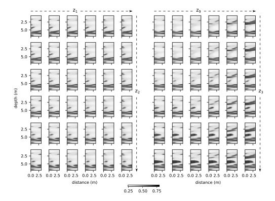
Figure 5.8: Examples of VAE latent traversals (stepping in two latent dimensions while keeping the rest fixed) for: latent dimensions  $z_1$  and  $z_2$  (left) and latent dimensions  $z_9$  and  $z_3$  (right). The colorscale is with respect to the model variable m prior to its transformation to velocity values.
