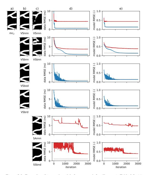
Figure 3.8: Examples of inverted models for  $mc_2$  truth for all cases in Table 3.2: (a) truth model, (b) accepted models according to defined threshold, (c) rejected models, (d) data RMSE vs. iterations plots (blue for accepted models and red for rejected models and dashed line indicates defined threshold) and (e) model RMSE vs. iterations plots (dashed line indicates model RMSE for encode-decode operation).
