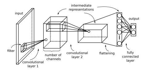
Figure 5.2: A sketch of a CNN depicting the general architecture and its main components.
