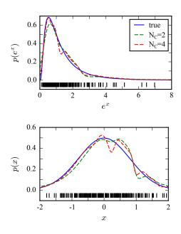
Figure 4.4: Comparison of the adaptive KDE for a non-linearly transformed space when the number of clusters is chosen by silhouette index ( $N_c$ =2) and by cross-validation ( $N_c$ =4). Vertical markers in the lower part denote the samples used to approximate the probability distribution. Both plots show the same samples, with the upper one representing an exponential transformation of the values in the lower one.
