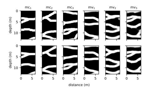
Figure 3.7: Truth models (first row): cropped from training image (denoted by "mc") and generated from trained VAE (denoted by "mv"). Corresponding models resulting from encode-decode of truth models (second row). Subindex indicates level of complexity, with "1" being the least complex.
