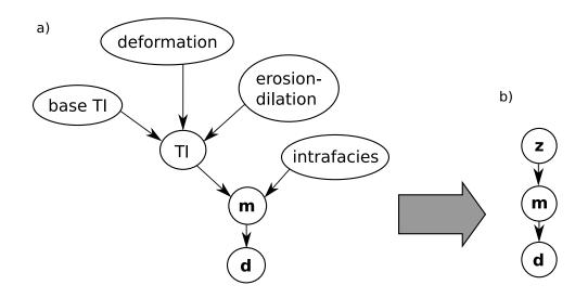
Figure 5.1: Probabilistic graphical models for: (a) the original variables which is used to train the VAE and (b) the latent variables (i.e. including the VAE) which is used for inversion. m, d and z refer to the model, data and latent vectors, respectively.
