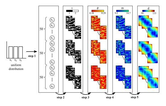
Figure 4.5: Sketch of the hierarchical sampling process for the geological scenario where s is the geological scenario index, t is the facies index,  $\phi$  is the porosity, m is the relative dielectric permittivity and d are electromagnetic wave traveltimes in nanoseconds plus added Gaussian noise with  $\sigma = 1.4 ns$ . Steps 1 through 5 are described in the text.
