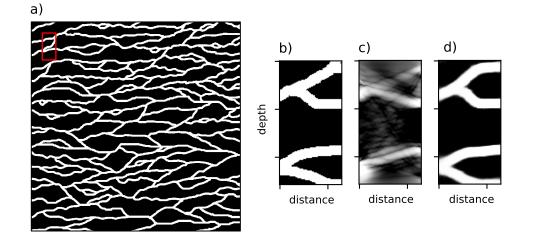
Figure 1.1: Inversion with prior information: (a) pattern samples for a highly structured subsurface in the form of a training image where the red rectangle shows the size of the domain of interest, (b) truth subsurface model, (c) inverted model with smooth regularization, and (d) inverted model with prior obtained from the training image.
