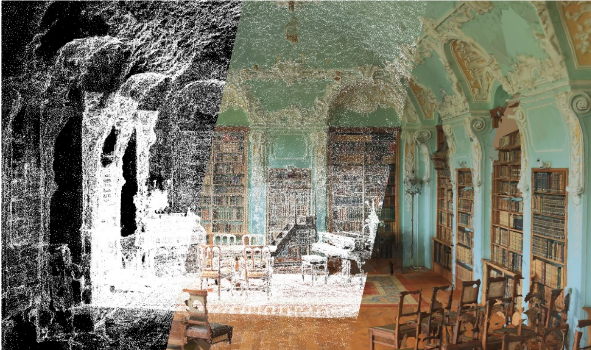
Example of a mesh generated from a 3D captured environment for a cool heritage project with Roman Robroek . (Left) 3D Point Cloud, (Middle) Vertices of the mesh overlay, (Right) Textured Mesh.
