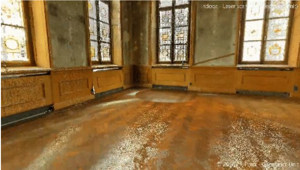
Real-time Multi-scale point cloud of different datasets captured and combined
