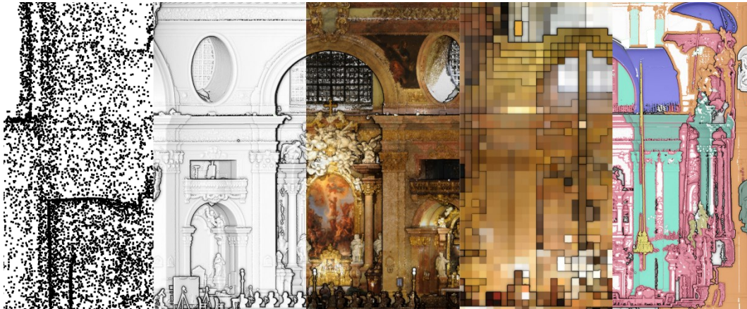
Different renderings of a point cloud. From left to right, raw point cloud, shaded, colored, voxelized, semantized
