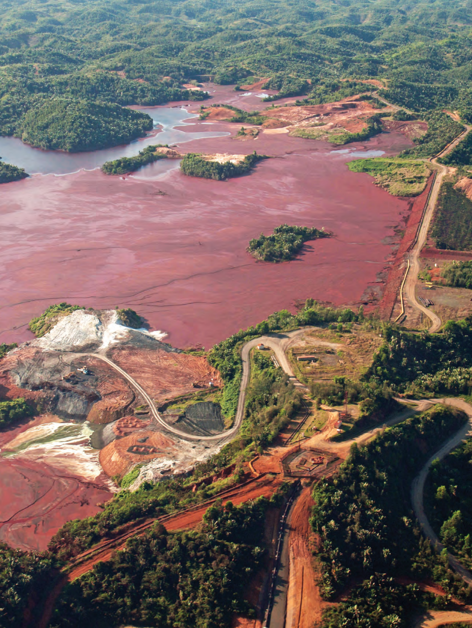
Mine tailings reservoir in Madagascar, receiving slurry through a pipeline from an ore processing plant. Photo: Roel Sloopweg © Shutterstock
