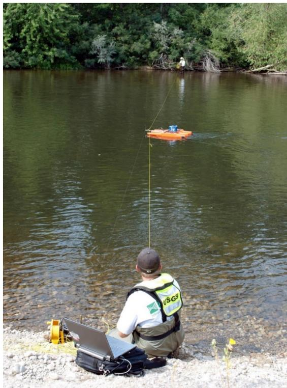
*Figure 2: Velocity measurement using ADCP (source: Tim Merrick, USGS)*
