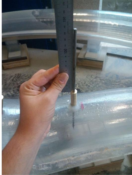
*Figure 85: Measurement of the distance of penetration of the shank*
