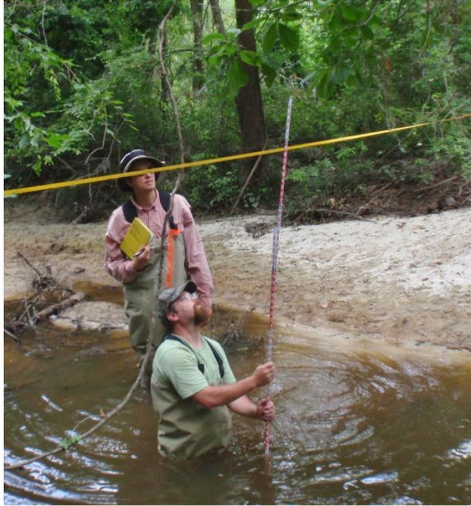
*Figure 1: Cross section measurement (source: [www.nuterinc.com](http://www.nuterinc.com))*
