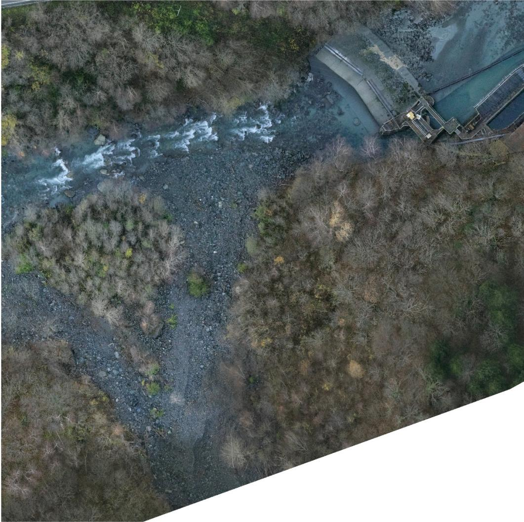
*Figure 6: The “cône de l’Infernet” provides sediments to the river Romanche in the French Alps (aerial view). The supply quantity and period depend on the winter season. This heavy sediment supply is prone to induce changes to the river morphology.*
