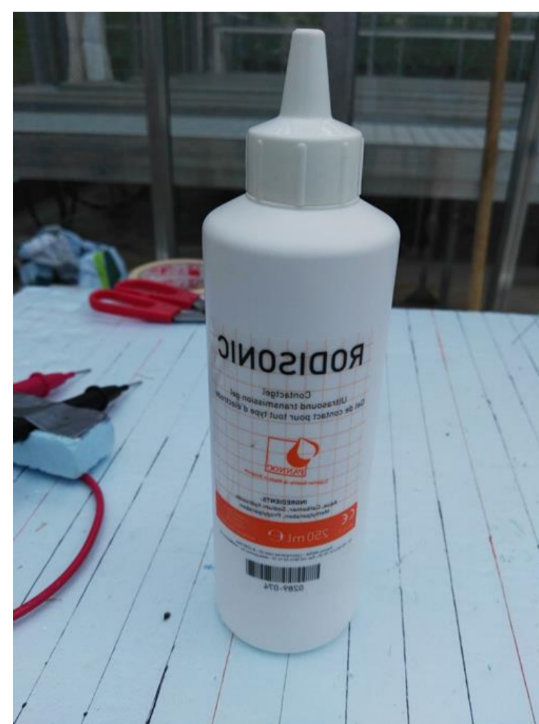
L-R: The growth media, experimental set-up and conductivity gel. The effect of contact resistance was minimized by the use of conductivity gel (Rodisonic, from pannoc Nv/SA Belgium)
