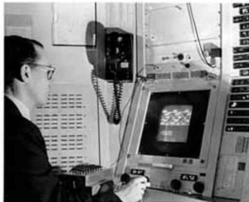
Figure 17 : "TX-2 Operating area-sketchpad in use" illustration 1.2 de Sketchpad : A man-machine graphical communication system (Sutherland 1963)
