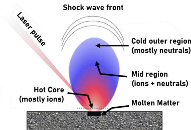
**FIGURE 3** Schematic illustration of laser-induced plasma. Adapted from Chaudhary et al. (2016) [Color figure can be viewed at [wileyonlinelibrary.com](http://wileyonlinelibrary.com)]
