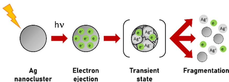
**FIGURE 2** Fragmentation of silver nanoparticle upon laser irradiation. The transient aggregate formed via the photoejection of electrons is considered as a precursor for complete fragmentation of the nanoparticle. Adapted with permission from Kamat et al. (1998). © 1998 American Chemical Society [Color figure can be viewed at [wileyonlinelibrary.com](http://wileyonlinelibrary.com)]
