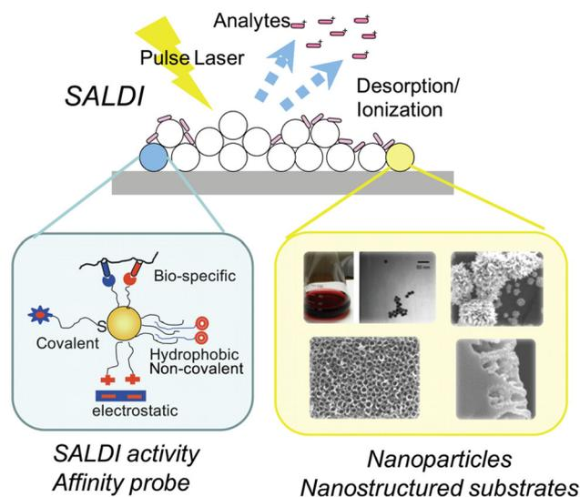
**FIGURE 12** Schematic representations of SALDI-MS using various nanoparticles and nanostructured substrates and an affinity probe. Reprinted with permission from Arakawa et al. (2010). © 2010 The Japan Society for Analytical Chemistry [Color figure can be viewed at [wileyonlinelibrary.com](http://wileyonlinelibrary.com)]
