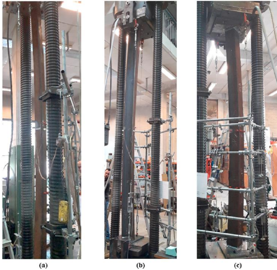
Fig. 15. Final deformed shape of (a) Sp15 with a pure flexural buckling mode, (b) Sp26 with a flexural-torsional failure buckling mode and (c) Sp14 with a mixed mode between flexural and flexural torsional buckling.
