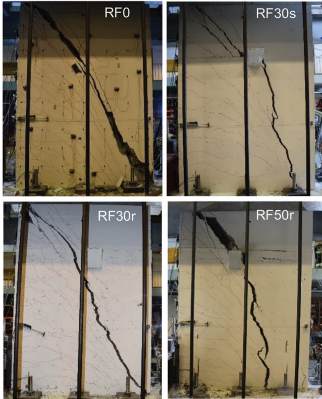
Fig. 13—Test specimens after failure.
