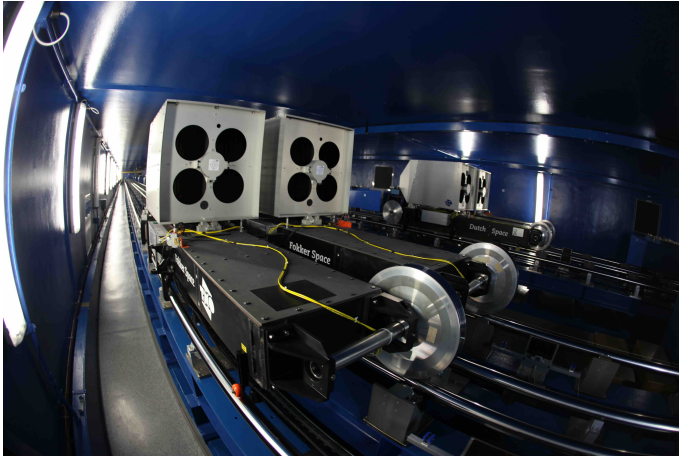
Figure 45. Zoom on one of the optical delay lines used in the tunnel of the VLTI at ESO, Paranal, Chile.
