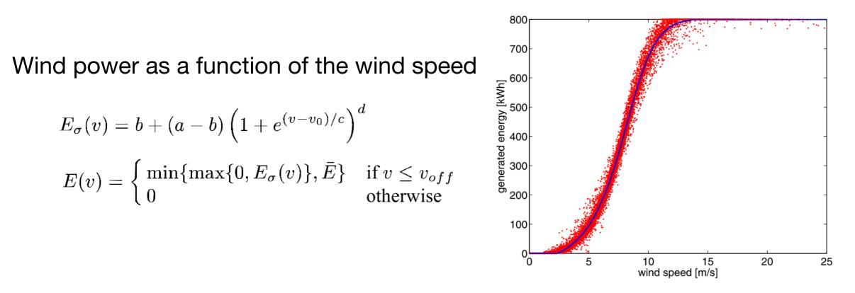
Fig. 3. Hourly generated energy vs hourly average wind speed for a 800 kW wind turbine (red points), and model (16) fitted to the data (solid blue curve).
