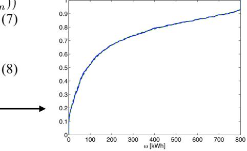
Fig. 2. Empirical *cdf* (solid) of the random variable  $w_{20}$  for a 800 kW wind turbine and corresponding BGM model (dashed) estimated from data. The two curves are in practice overlapping.
