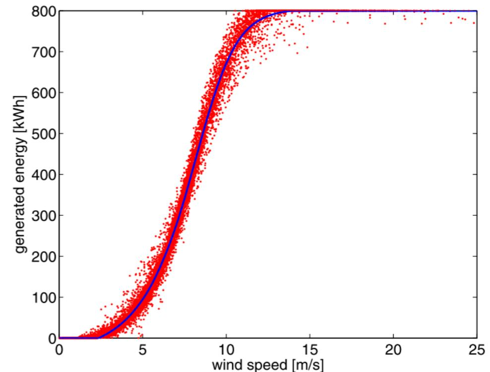
Fig. 3. Hourly generated energy vs hourly average wind speed for a 800 kW wind turbine (red points), and model (16) fitted to the data (solid blue curve).
