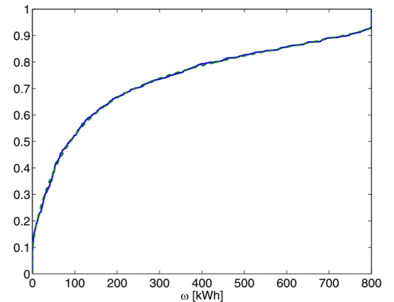
Fig. 2. Empirical *cdf* (solid) of the random variable  $w_{20}$  for a 800 kW wind turbine and corresponding BGM model (dashed) estimated from data. The two curves are in practice overlapping.
