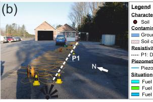
**Characterization points** • Soil • Groundwater (piezometer) • Pumping wells Contaminated areas Groundwater contamination (C<sub>10</sub>-C<sub>40</sub>>0.3 mg/l) Soil contamination (C<sub>10</sub>-C<sub>40</sub>>160 mg/kg) **Resistivity profiles** ---- P1: Dipole-Dipole array (48 electrodes - spacing 1 m) Piezometrv Piezometric levels in metres above sea level Fuel Tank 12000 L 📖 Hangar Road Dirt road Fuel Tank 20000 L Sidewalk Parking Fuel Tank 42000 L Parcel
