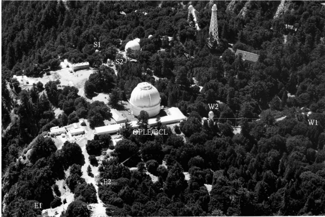
Figure 2.2: Picture of the CHARA Array taken from the North looking South. The six 1 m telescopes are identified by their name, as well as the Optical Path Length Equaliser and Beam Combination Laboratory (OPL/BCL).
