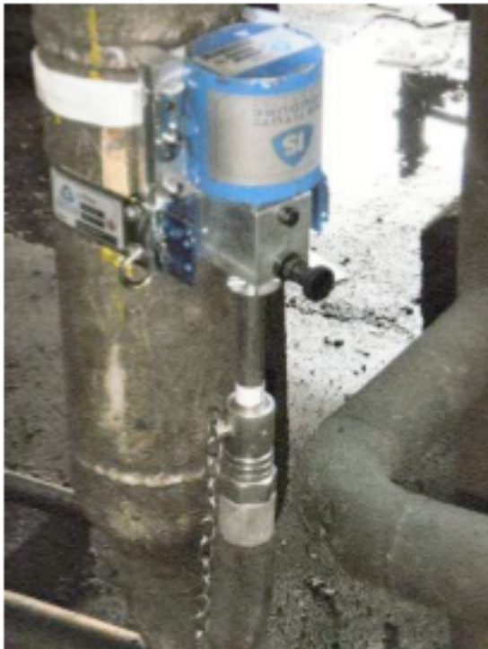
Figure 38 – The “γ-Prox” in control situation of a welding pipe inspection
