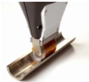
Figure 45 – EC flexible array probe adapted to the inspection of curve shaped surface.
