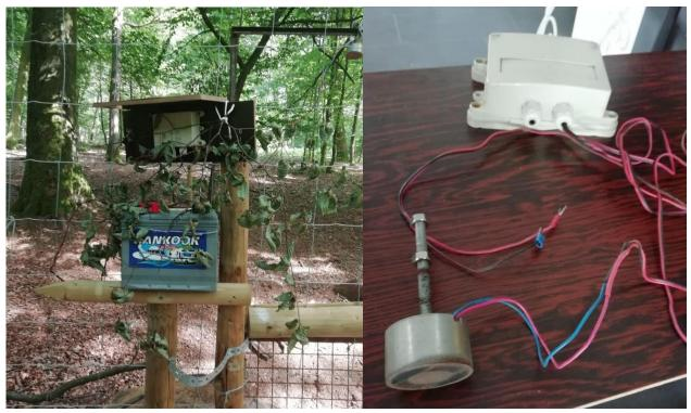
Figures 10 et 11 – Left: the remote triggering system installed in the field (battery, housing and magnet). Right: the box in charge of remotely breaking the current and thus the magnetic field of the magnet.
