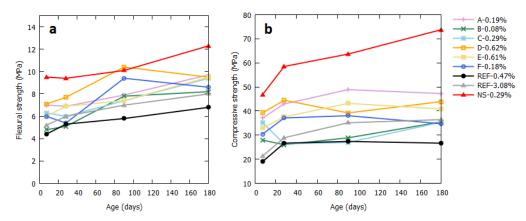
Figure 5. Flexural (a) and compressive (b) strength of the mortar samples after 7, 28, 90, and 180 days.
