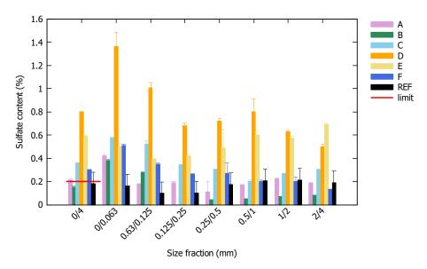
**Figure 2.** Water soluble sulfate content of the FRA in total and per size fraction.
