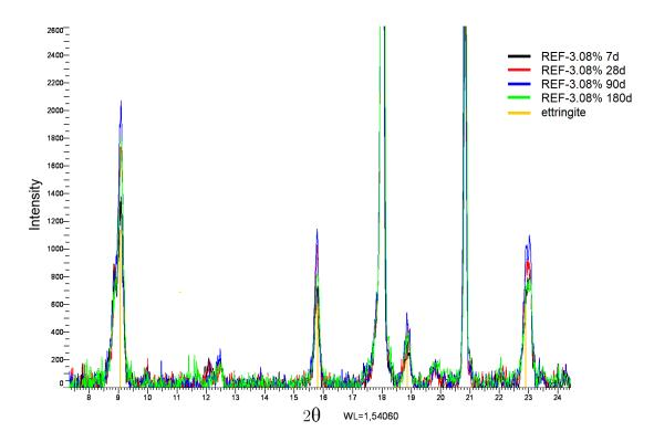
**Figure 4.** XRD analysis of "REF-3.08%" at 7, 28, 90, and 180 days.
