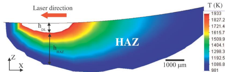
Fig. 10. Temperature distribution within the fusion zone and the HAZ in a longitudinal section located in the middle of the substrate at t = 22.7 s (i.e. half of the first layer deposition), showing the asymmetrical thermal gradient.
