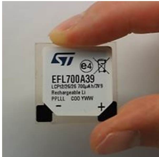
Figure 4. Example of microbattery developed during EnSO project.
