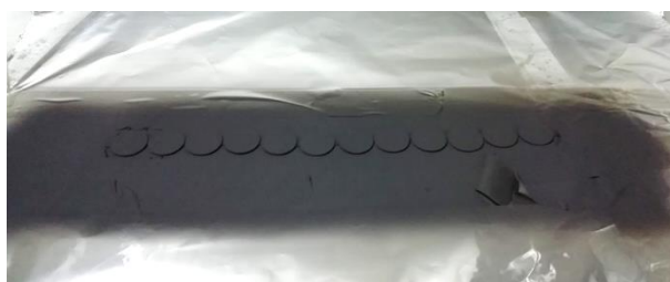
Figure 4.14. \text{LCO}_{\text{TiO}_2} -LLZO 30% deposited on stainless steel disc.
