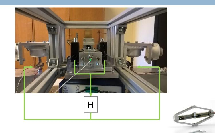
Controller H : 4 Lags, 1 High-Pass filter and 1 Lead
