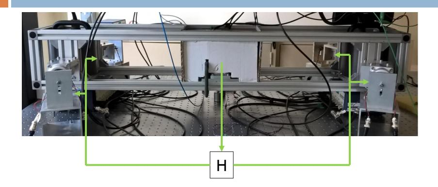
Controller H : 4 Lags, 1 High-Pass filter and 1 Lead The same as in the previous experiment
