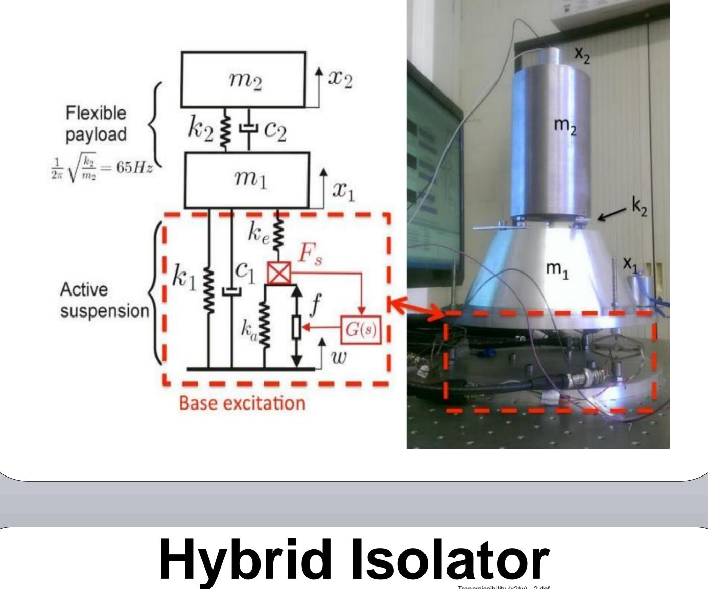
payload is reduced by up to a factor of 5. This effect is broadband, not only at the resonance frequencies
