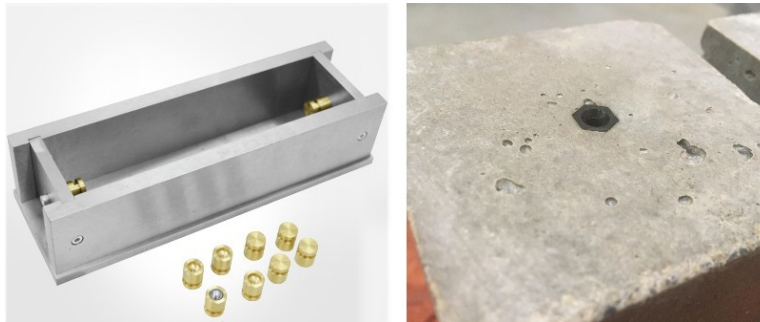
Figure 6.1: To register the length of a mortar or concrete sample with a length comparator, measuring studs need to be placed into the bars during fabrication.
