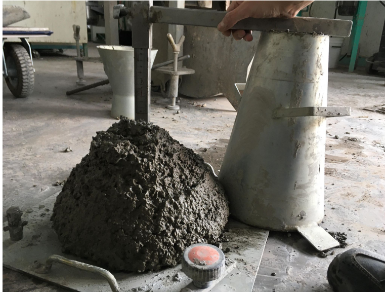
Figure 5.2: Testing the slump of a concrete mix with an Abrams cone
