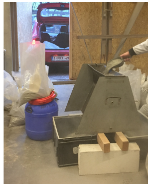
Figure 4.2: The homogenization process of the 2 obtained FRA fractions, with the help of a riffle splitter.
