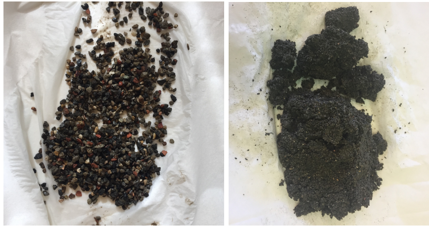
Figure 4.6: Determination of the SSD state according to method n°78 by IFSTTAR, for the size fractions 2/4 and 0.5/1 mm respectively. The smaller the particle size, the more difficult it gets to measure the SSD state accurately.
