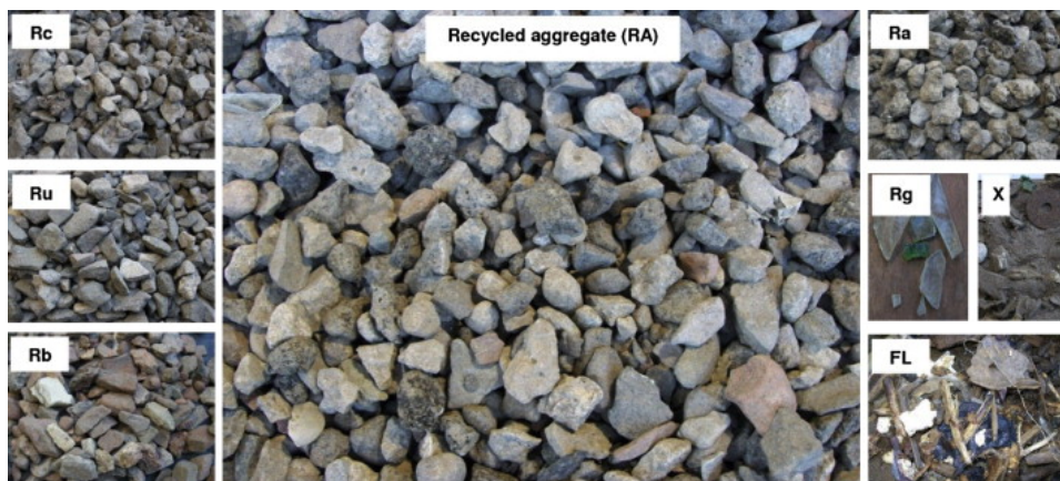
Figure 1.3: The different constituents used in the classification of RA (from EN12620 [32]) and their physical appearance (from Medina et al. [34]).
