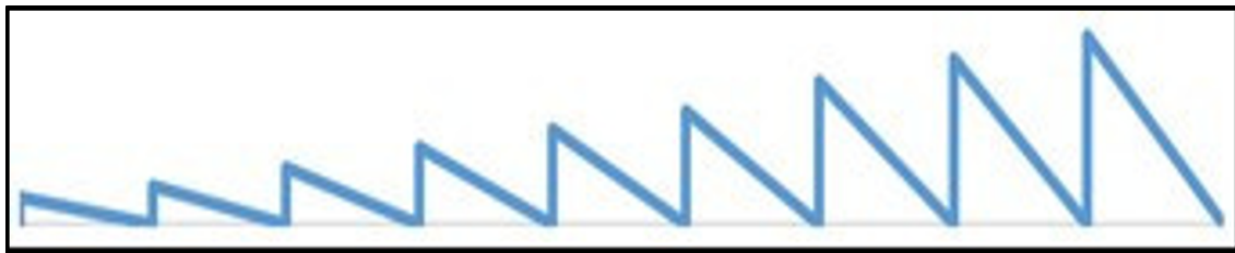
Figure 4 : Example of multi-blaze grating. The period remains constant. The blaze angle is variable and the groove depth is adapted.
