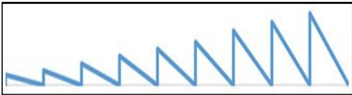
Figure 3 : Example of multi-blaze grating. The period remains constant. The blaze angle is variable and the groove depth is adapted.
