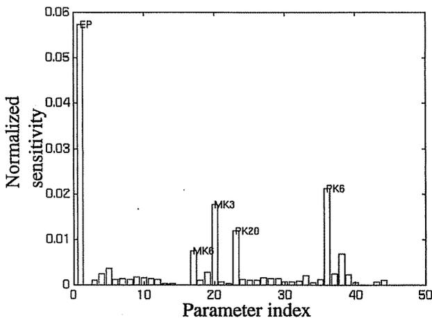
Fig. 6. Sensitivity analysis for the correlation (MAC) of the first experimental mode
