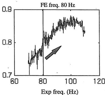
Fig. 5. FDAC correlation at FE 80 Hz
