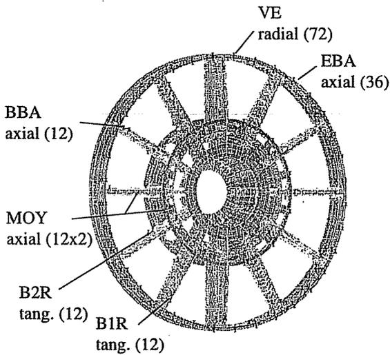
Figure 3. The fan frame and the actual sensor configuration
