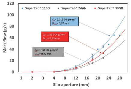
Figure 3: Mass flow rate versus aperture for powders.
