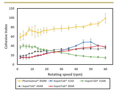
Figure 4: Cohesive index versus rotating drum speed. Shear-thickening behaviours are observed, except for powder SuperTab<sup>®</sup> 21AN, which exhibits strong shear-thinning behaviour.
