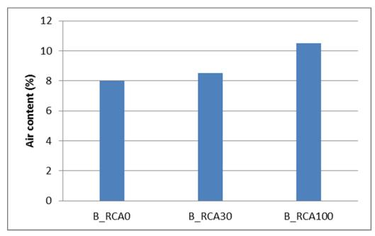
The air content of concrete increases when the substitution of recycled aggregates increases
