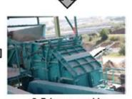
5. Primary crushing (Impact crusher)
