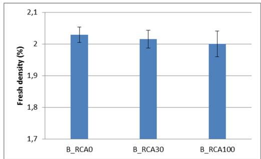
The density of fresh concrete slightly decreases when the substitution of RCA increases
