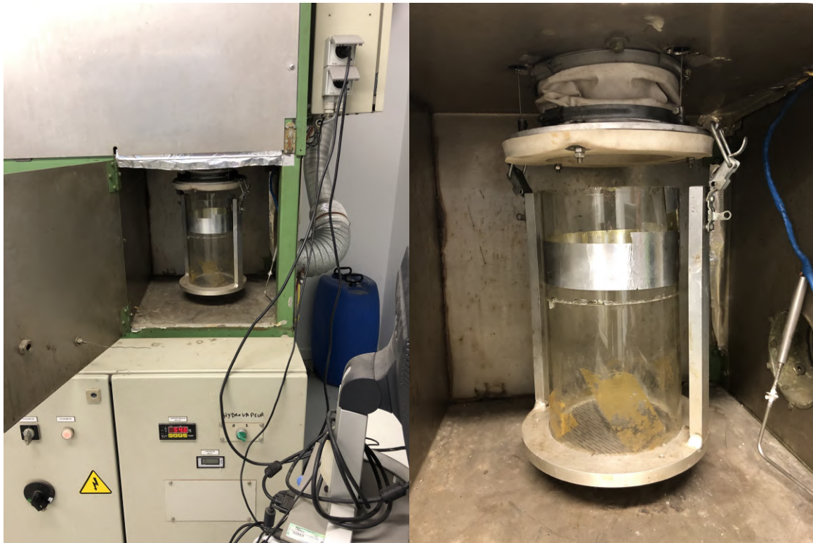
Figure 5.10: Macro-dryer used for the convective drying experiment, with the cell containing the sample.
