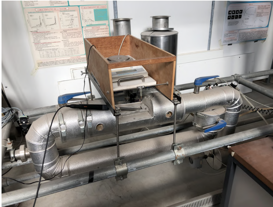
Figure 5.7: Convective dryer (called micro-dryer) built by A. Léonard during her PhD thesis [ Léonard, 2002 ]
