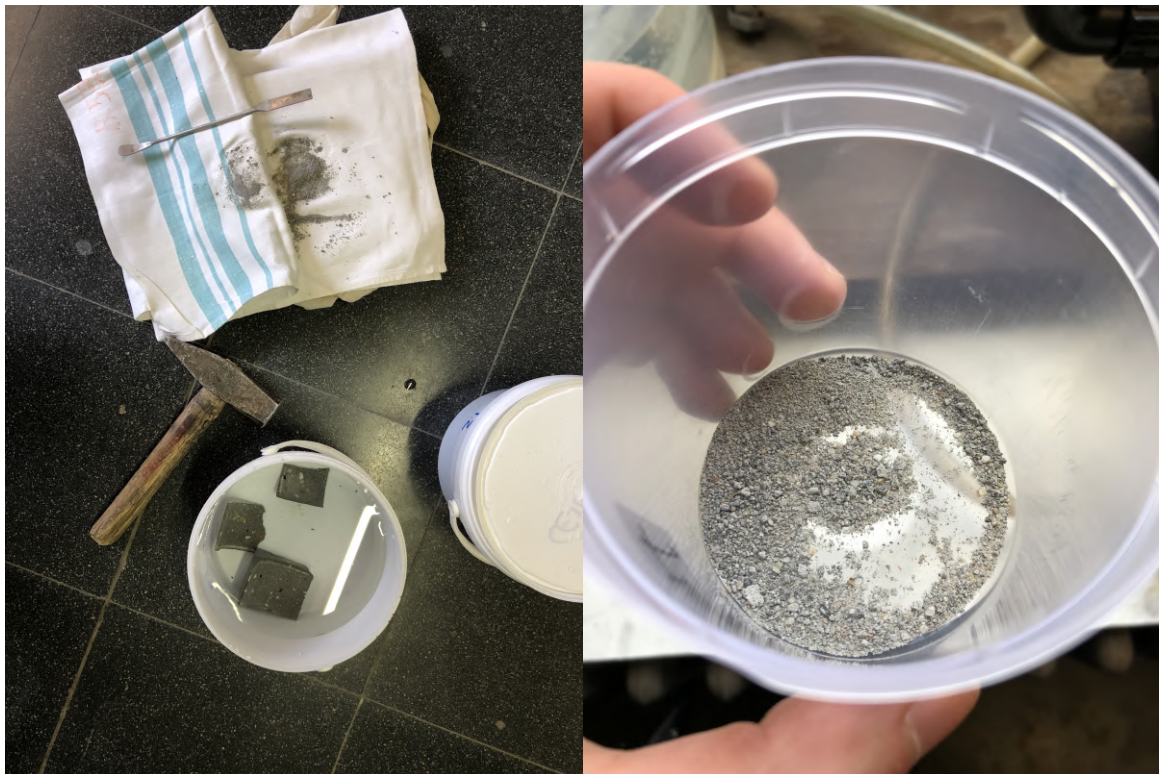
Figure 5.6: Crushing process and final sample for the DVS Intrinsic.
