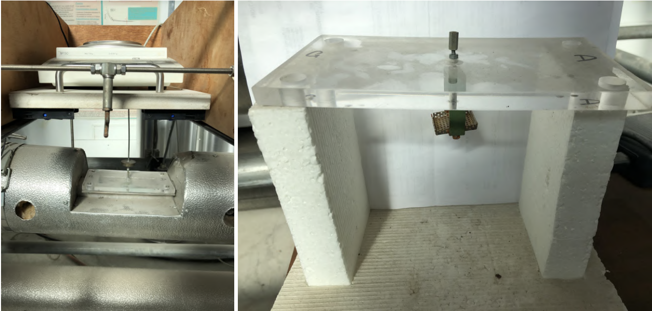
Figure 5.8: Platform and support containing the sample.
