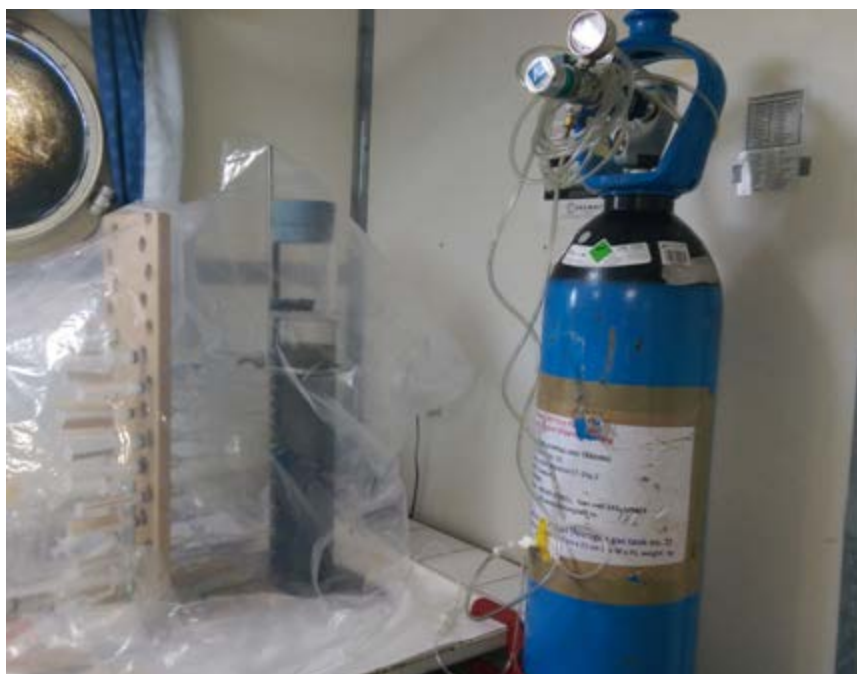
Figure 2.5. Schematic diagram of Rhizon and its periphery (top panel) and picture of the setup for porewater extractions using Rhizons (bottom panel).
