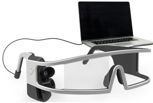
Figure 7.2: The figure shows, our data collection system, consisting of a pair of eye-glasses (conceived by our team) linked to a computer used to acquire the images of one eye and to automatically produce a validated LoD signal.
