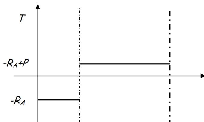
$$T = \frac{dM}{dx} = \begin{cases} +R_A & \text{si } x \leq L_1 \\ +R_A - P & \text{si } x > L_1 \end{cases}$$
