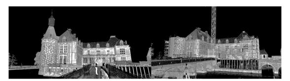
**Figure 3.** TLS intensity-based rendering of the point cloud of the castle acquired before the renovation in February 2016 (**left image**), and in April 2019 during the renovation (**right image**).
