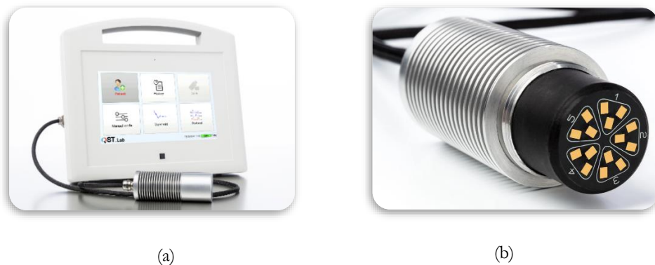
Figure 1.5. The thermal cutaneous stimulator (TCSII). (a) Control unit and stimulation probe. (b) Stimulation probe. The 5 stimulation surfaces that can be activated separately are delimited by white lines and labeled. (From QST lab website [qst-lab.eu], with permission of André Dufour)
