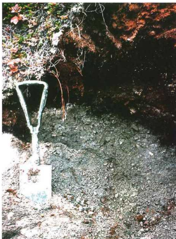
Figure 3. Aggregates of silts just below the peat in the palsa shown in Figure 4. These very highly compacted angular lumps of silt are a cryostructure due to the formation of segregation ice.
