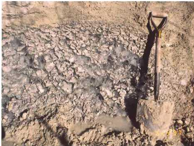
Figure 3. Aggregates of silts just below the peat in the palsa shown in Figure 4. These very highly compacted angular lumps of silt are a cryostructure due to the formation of segregation ice.
