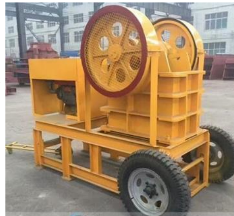
Figure 11 : Jaw crusher (Gorlé and Saeys, 1991) Figure 12 : (JXSC jaw crusher, 2018)
