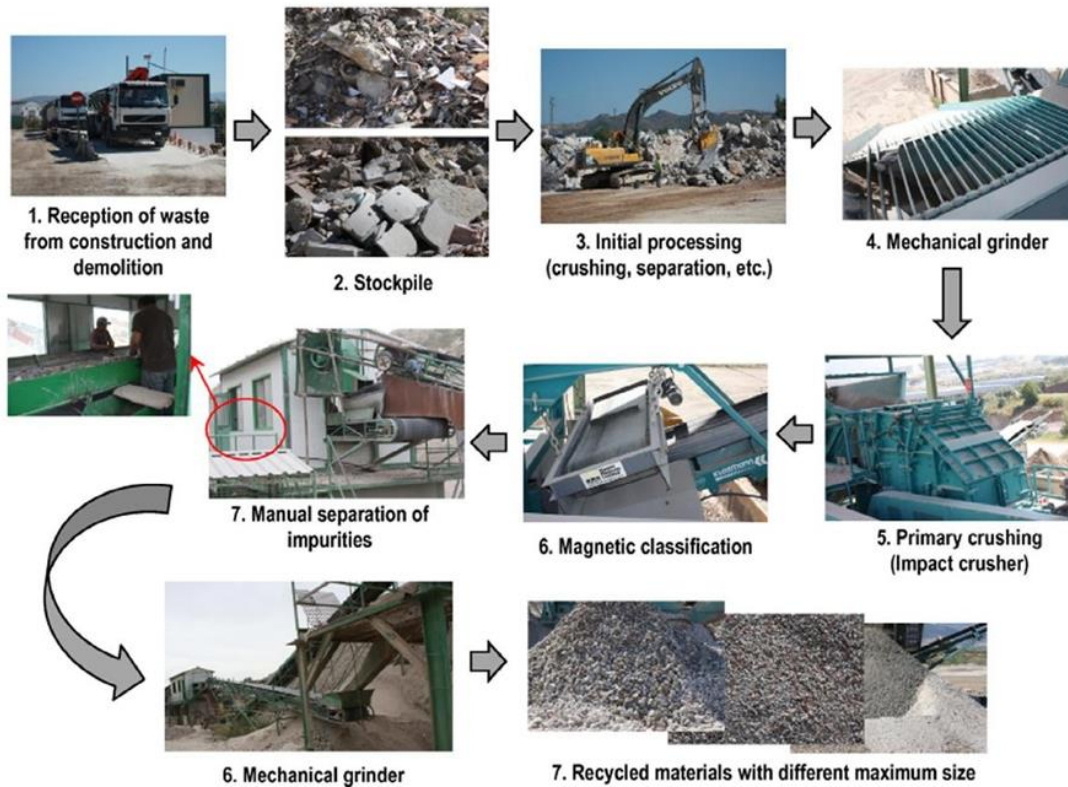
Figure 17: C&DW recycling process (source: (Medina et al., 2015))
