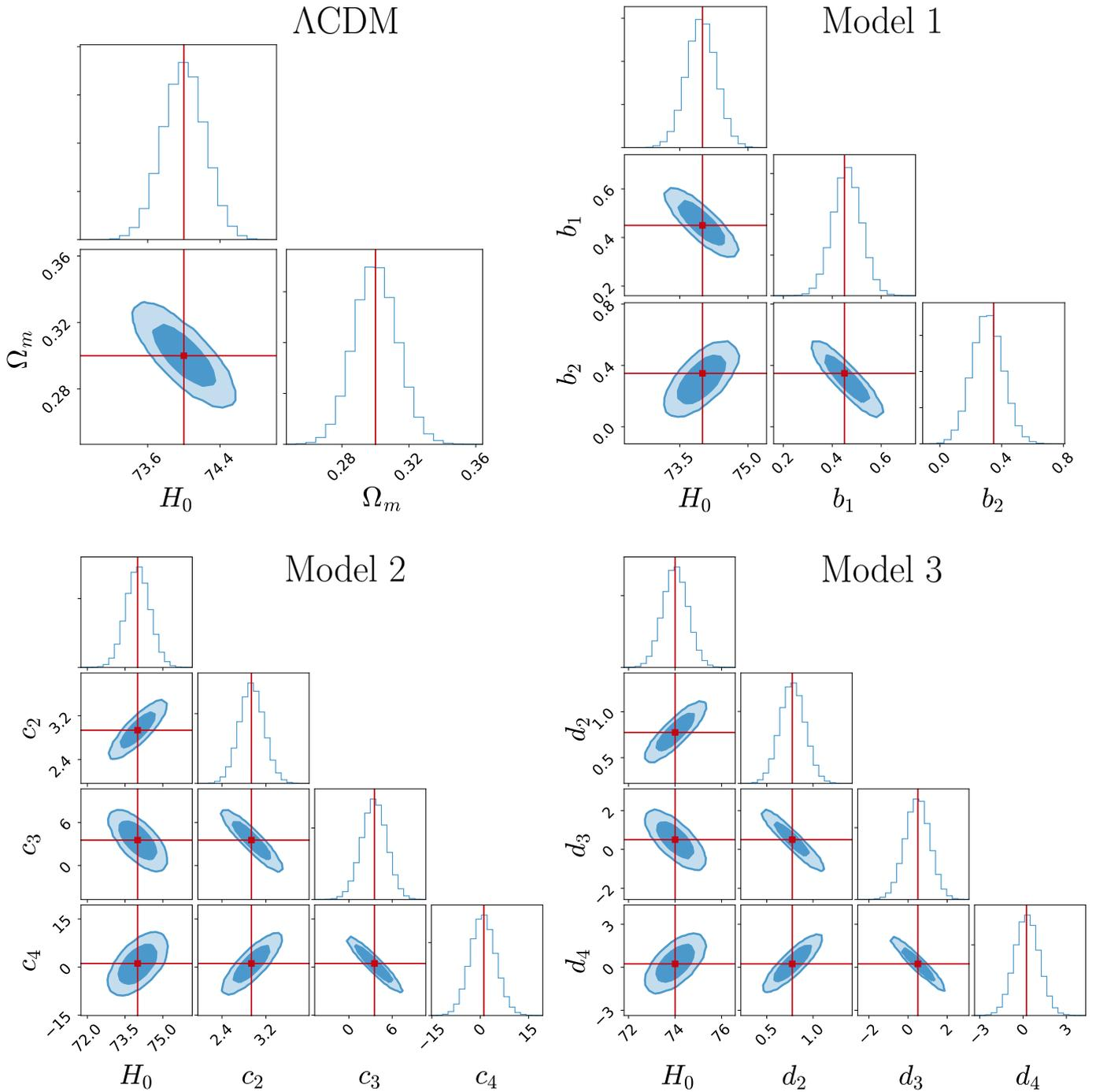
**Fig. B.2.** Best-fit values of flat  $\Lambda$ CDM and polynomial parametrisation models 1-3 to mock data. The mock data is generated by replacing the Pantheon distance modulus points by their fiducial flat  $\Lambda$ CDM values. The red lines indicate the canonical  $\Lambda$ CDM values of  $\Omega_m$ ,  $H_0$  and the expansion coefficients  $b_i$ ,  $c_i$ , and  $d_i$ .
