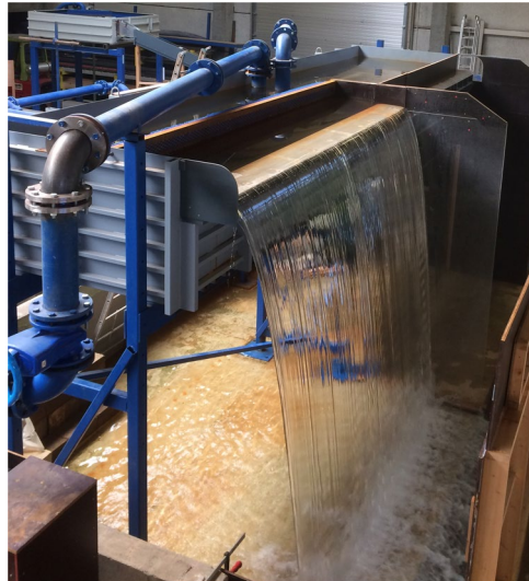
Fig. 2 Model 1- View of the prototype scale model with flow over the unconfined weir.
