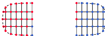
Figure 6.5: Representation of the distribution of the nodes on the MPI processes without overlaps. The nodes of the overlaps of Fig. 6.4 are distributed among the MPI processes in order to have a Map of nodes which is 1-to-1.
