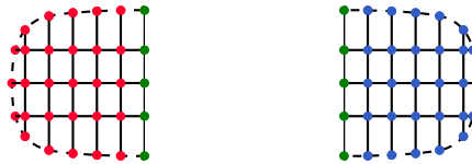
Figure 6.4: Representation of the distribution of the nodes on the MPI processes with overlaps. As the nodes on the interface of the mesh partitions are shared between at least two MPI processes, we create a Map of nodes which includes the overlaps. The nodes in green are the nodes of the overlap. Those nodes are stored in the memory associated to each MPI process.
