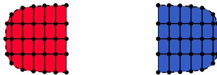
Figure 6.3: Representation of the distribution of the elements on the MPI processes. The elements of a mesh partition are associated to one MPI process.
