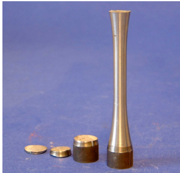
Figure 6: Multiple section fracture on a sample after fatigue test
