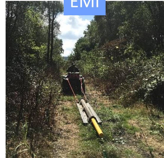
Mobile survey with DUALEM-421S: sampling rate 5 Hz, avg. driving speed 8.6 km/h, avg. sampling interval 0.5 m
