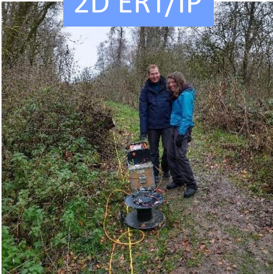
ABEM Terrameter LS: 64 electrodes at 3 m spacing
