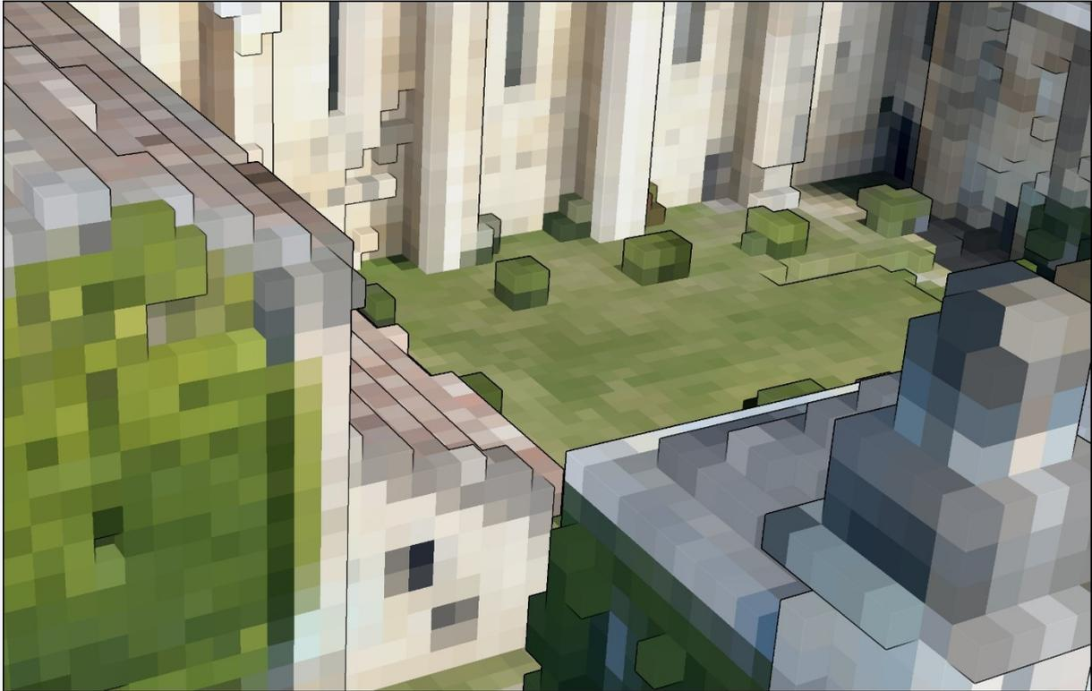
Example of voxel generalization based on an octree subdivision of the space occupied by the point cloud data.
