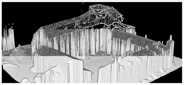
From top to bottom: The vertices of the mesh; the edges linking vertices together; the faces filling formed by vertices and edges, mostly triangular.
