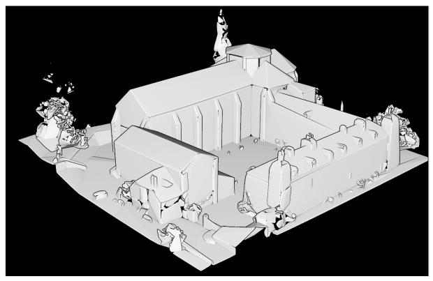
This is an automatically generated CAD model without a topology fix.
