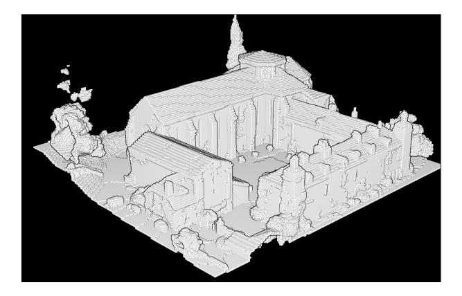
In the case of point cloud data, one can represent each point as a voxel of size , to get a "filled" view of empty spaces between points. It is mostly associated with data structures such as octrees, and permit to average a certain amount of points per voxel unit depending on the level of refinement needed (see example in the image below). This is very interesting, and I will cover the theory as well as the implementation in another dedicated article.
