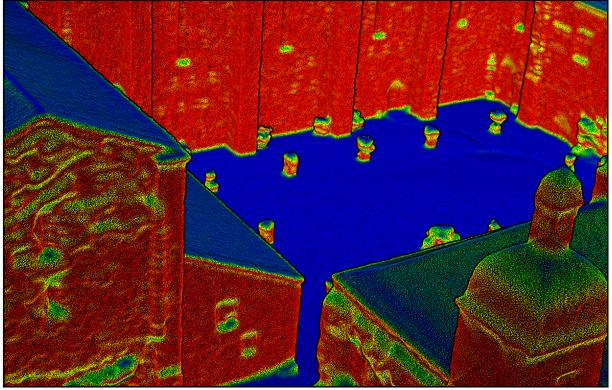
Color-based visualization of the verticality feature extracted to characterize the point cloud
