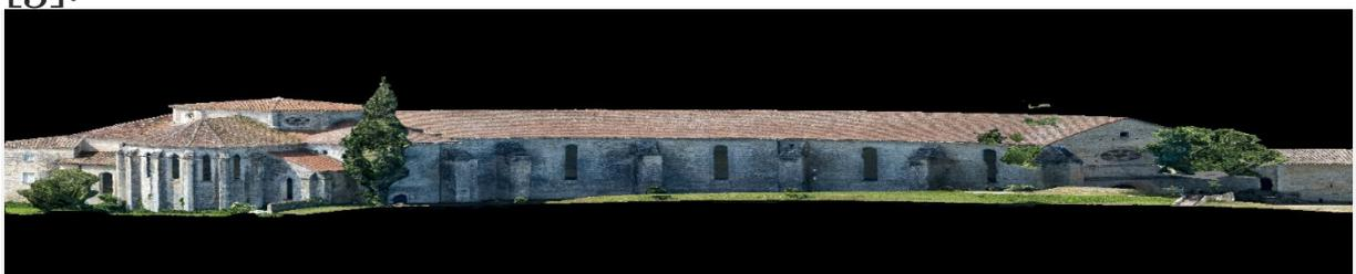
Example of widely deformed cylindrical projection of the point cloud
