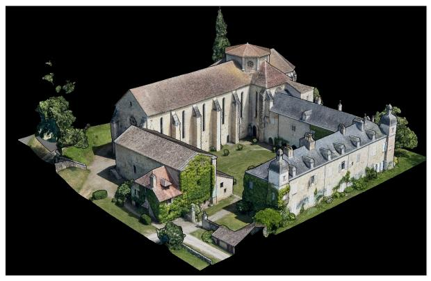
A 3D Point Cloud of an Abbey acquired in 2014 using photogrammetry (Gerpho), next to my hometown in the South of France 🙂. The Resolution is 1 cm, expressed as the Ground Sampling Distance.
