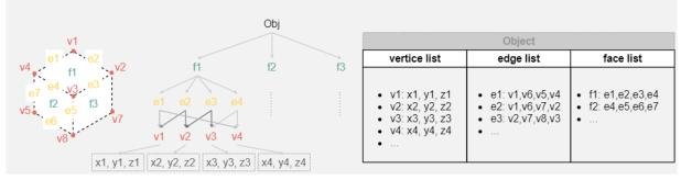
The schematization of the boundary representation underlying structure
