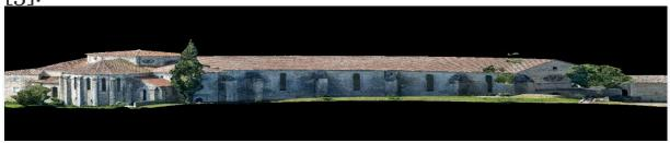
Example of widely deformed cylindrical projection of the point cloud
