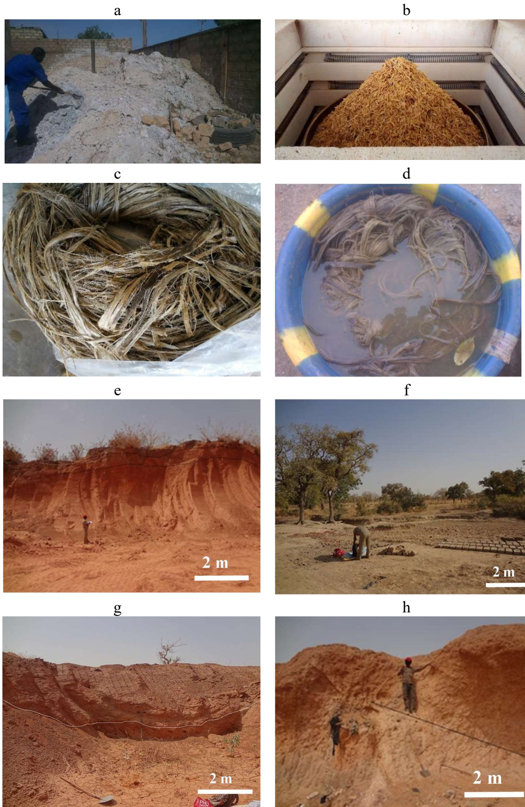
Figure 2.1. (a) collection of CCR, (b) calcination of rice husk, (c)-(d) retting processing of fibers, (e) clay materials in Kamboinse, (f) Pabre, (g) Kossodo, (h) Saaba
