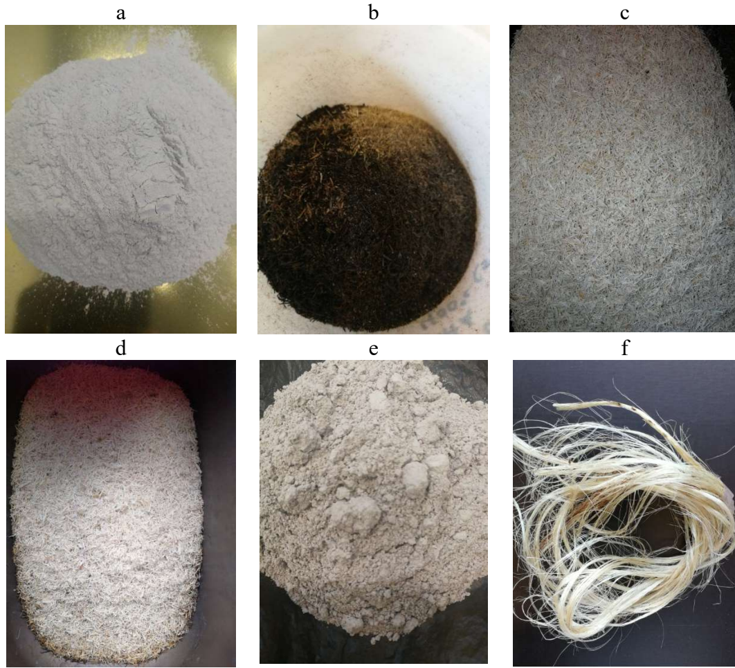
Figure 3.1. Processed materials (a) CCR, (b) calcined RHA (400 °C-4h), (c) RHA (500 °C-2h), (d) RHA (600 °C-1h), (e) ground RHA (500 °C-2h), (f) Okra bast fibers
