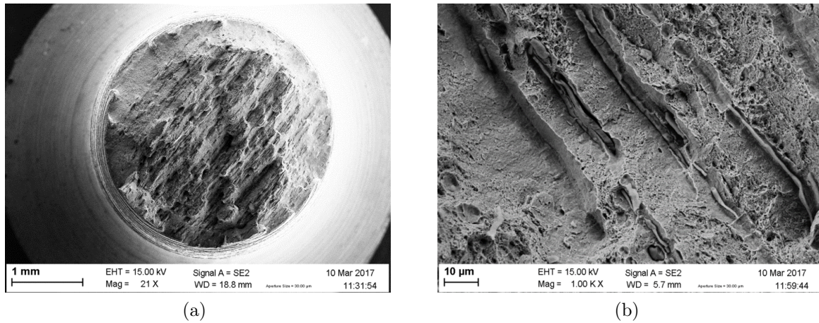
FIGURE 4.8: SEM pictures of the failure surface for a smooth round bar in the perp. direction. (a) General view. (b) Zoom on the central part.
