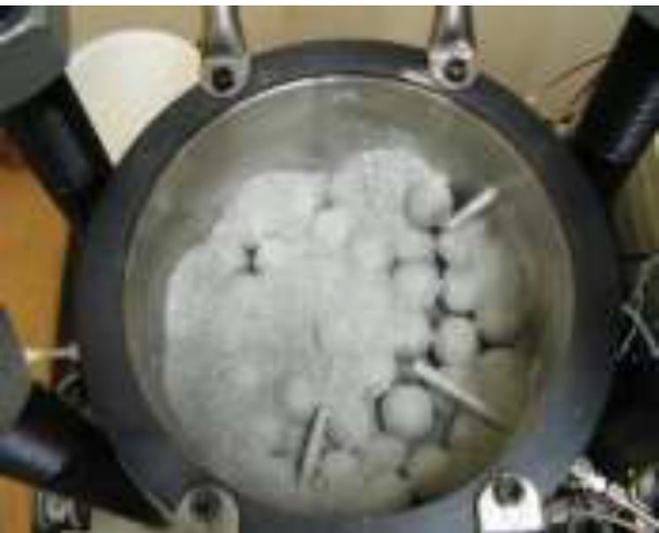
Second layer with crushed pellets during installation
