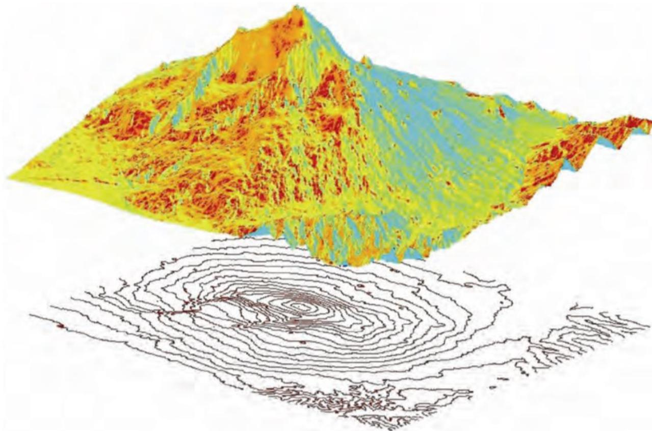
*Figure 2-6: Perspective view of Mount Etna as seen from the Northeast. The DEM of Mount Etna has been generated by unwrapping and re-sampling the flattened interferogram of Figure 2-5: The estimated vertical accuracy is better than 10 metres. Contour lines are shown below the DEM.*
