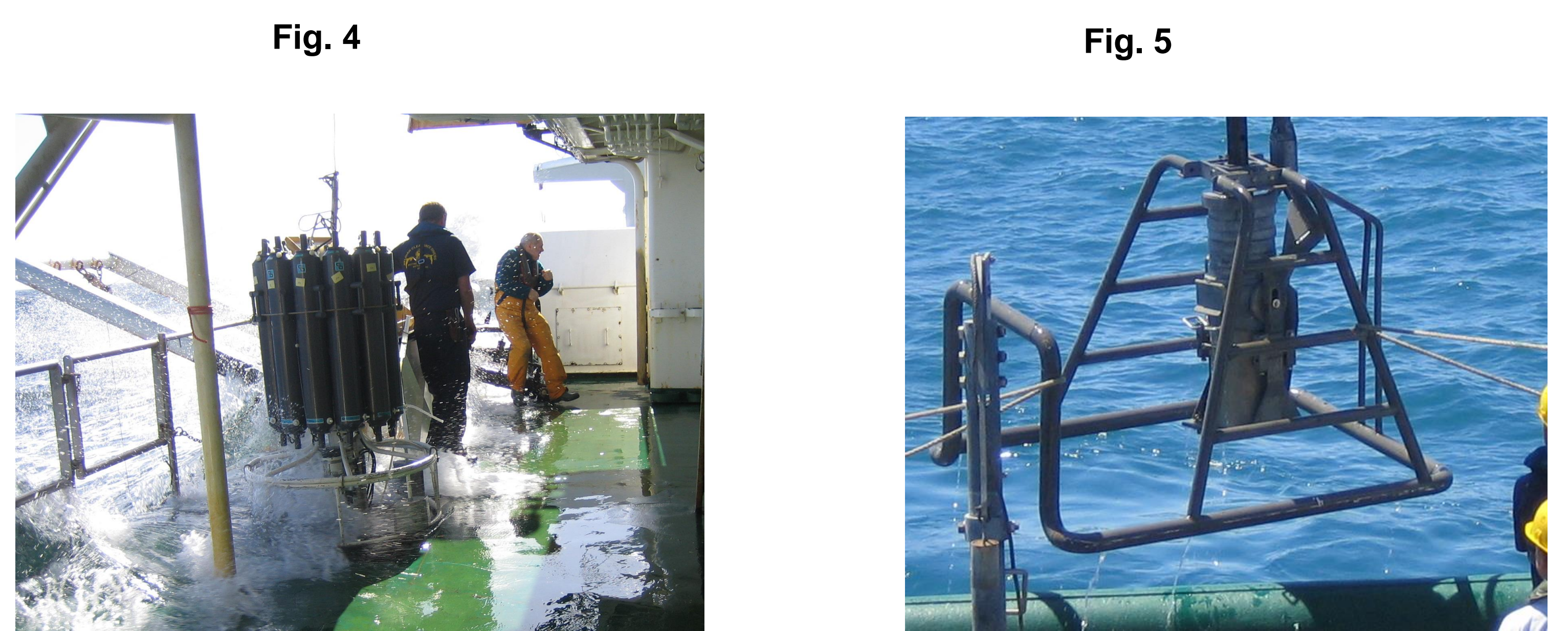
Figure 4: Rosette of 12 Niskin bottles. Figure 5: Boxcorer.
