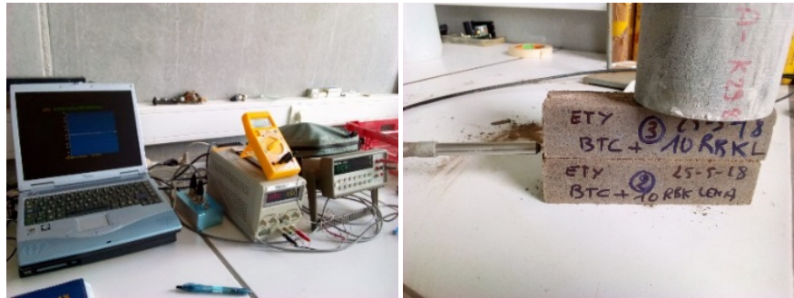
Figure 7. Measurement of thermal conductivity of CSEB after 14 and 28-days cure.
