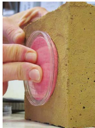
Figure 9. Sponge contact test principle [14].
