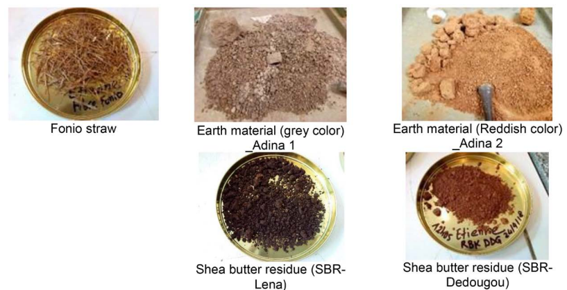
Figure 1. Earth material and stabilizers specimens.
