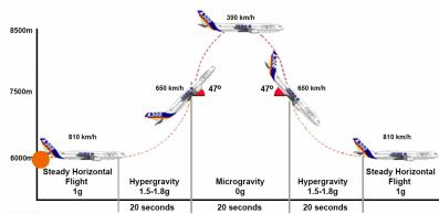
Parabolic flight trajectory
