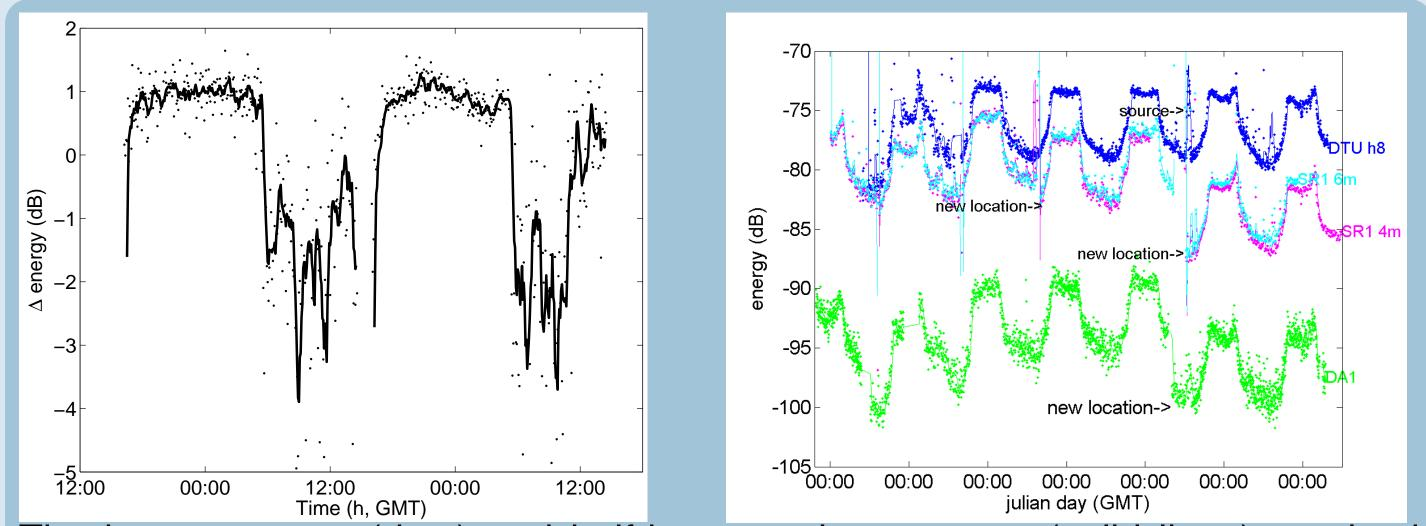
The instantaneous (dots) and half-hour moving average (solid lines) received energy from the transmitted signals (left panel) or environmental noise (right panel) show a diurnal pattern, where the energy sudden decreases at sunrise and increases at sunset.
