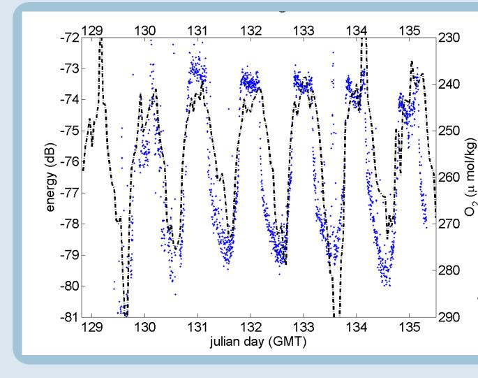
The comparison between the changes in dissolved O2 and the changes in noise power shows a high correlation. At sungrise the high gradient of change occurs earlier in acoustic data than in dissolved <sup>o</sup>O2, what could suggest that the air in plant tissues (aerenchymas) plays a major role in the acoustic signature of photosynthetic activity.
