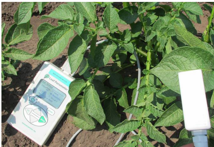
Measurements with the leaf porometer to determine stomatal conductance.
