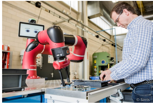
Figure 1.1: Sawyer, a collaborative robot from Rethink Robotics, Hahn group (picture from http://www.made-in-europe.nu/2017/05/erst-sawyer-cobot-met-ce-goedkeuring-in-de-benelux/ ).
